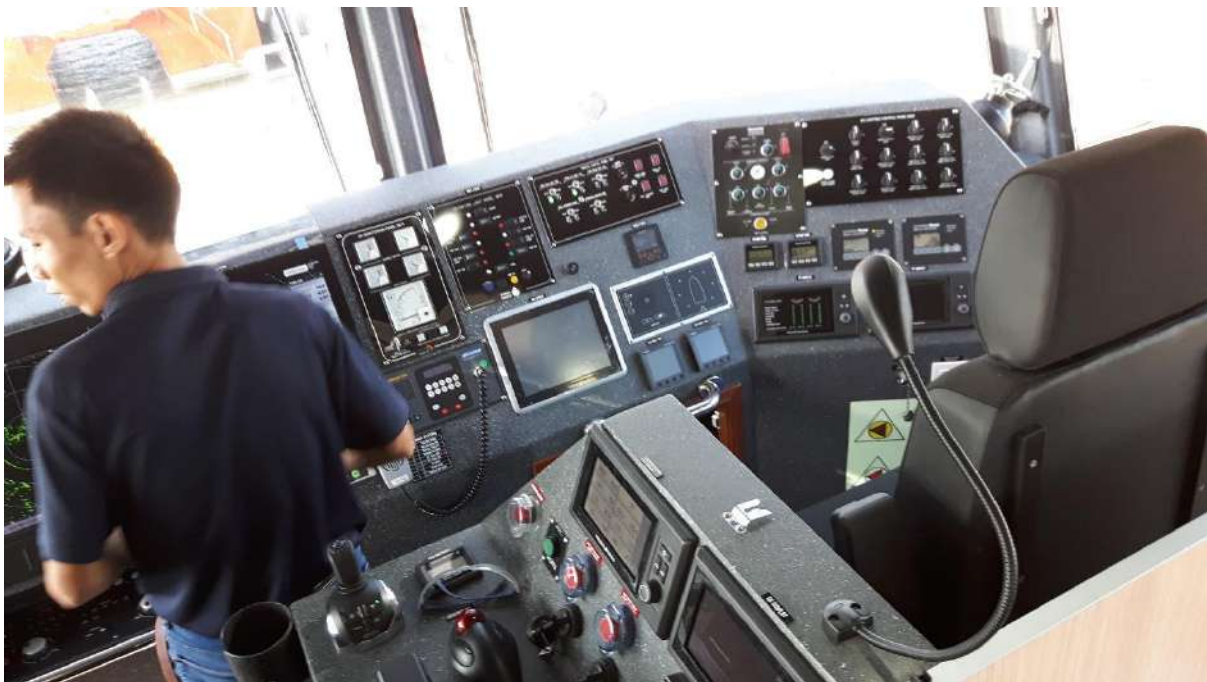
Photograph of bridge front. The engineer's seat is to starboard, the Master's seat out of shot at the left-hand corner, the Masters console centre bottom with the VHF radio just out of shot.
