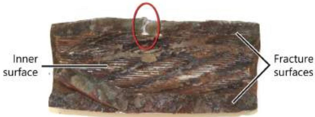
Figure 12. Inner surface and fracture surfaces of the broken aft starboard crimp sleeve, as well as a small region of fresh fracture (circled) (Source: TSB)
