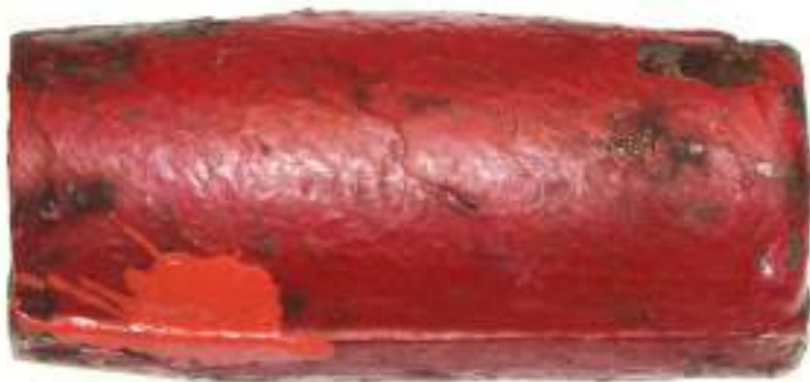
Figure 10. Broken portion of aft starboard crimp sleeve from upper end of sling (Source: TSB)
