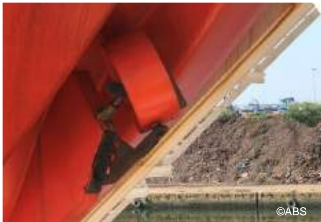
Free fall lifeboat hydraulic system for rudder malfunctioning
