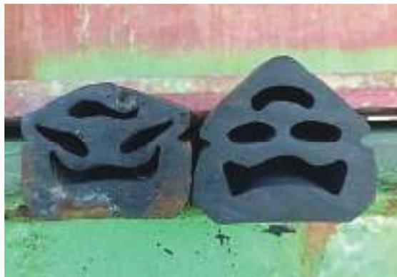
Photograph 9 Overcompressed CAT seal
