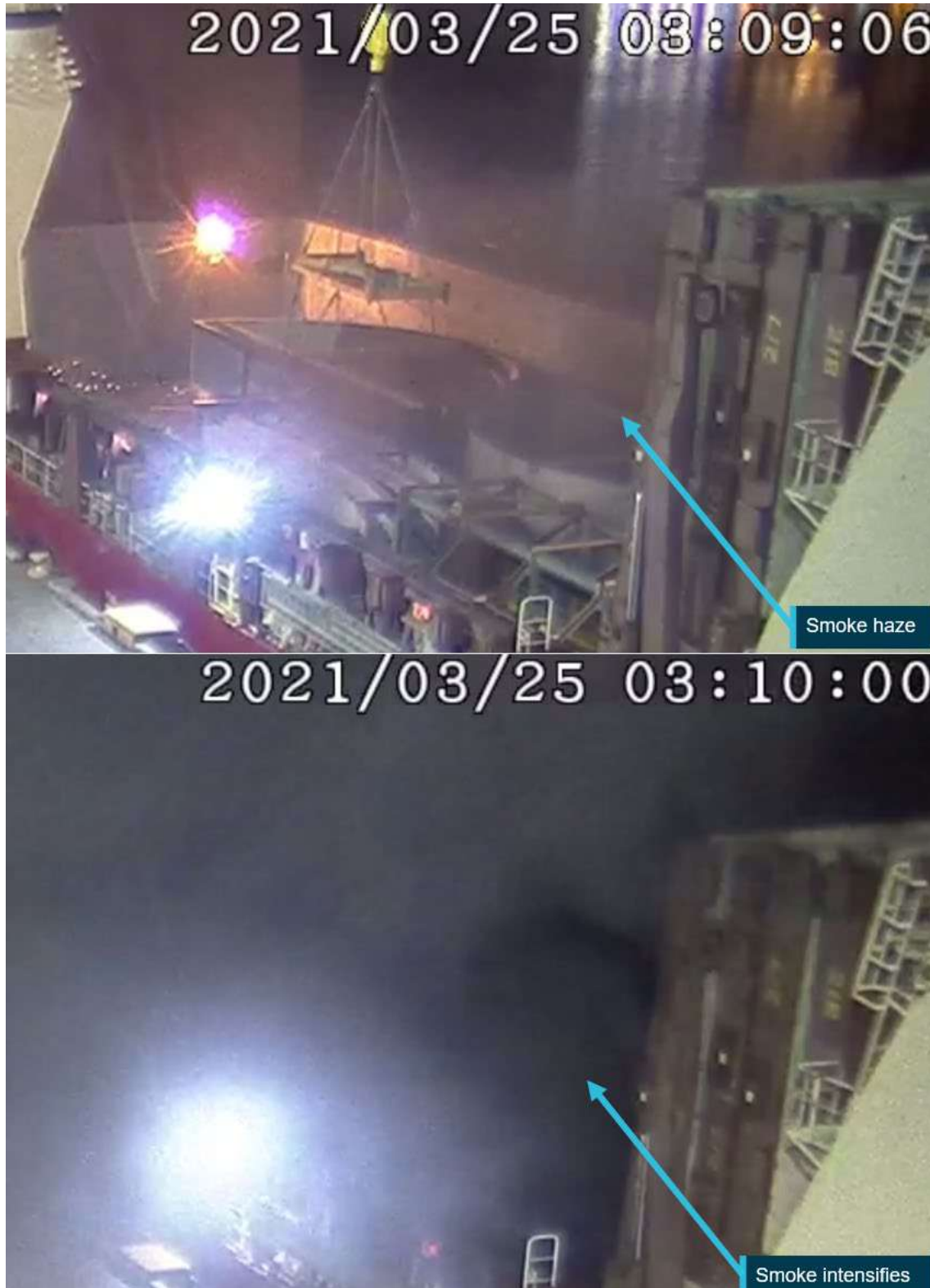
Figure 4: Intensifying smoke from the lower hold (CCTV frames at 0309 and 0310)
