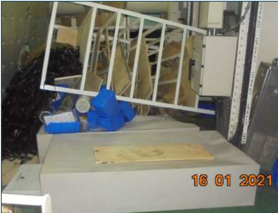
Figure 13: Overturned storage racks Source: Maersk A/S
