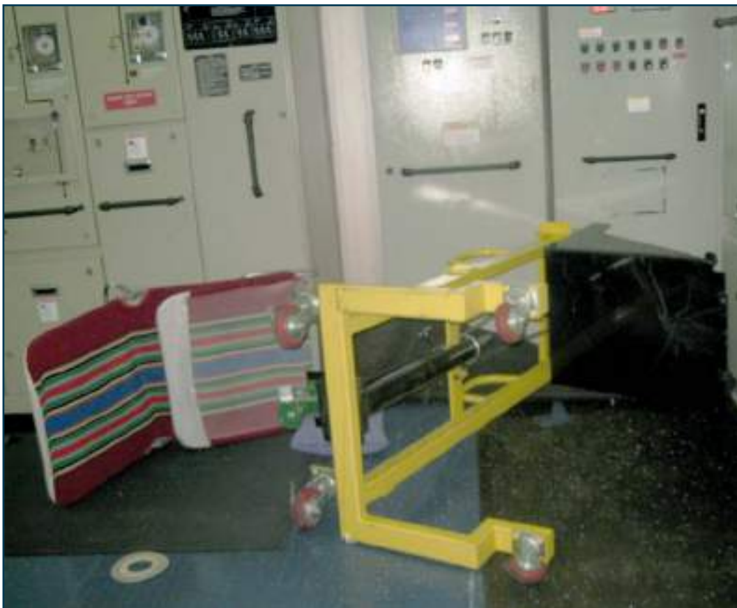
Figure 14: Overturned and displaced lifting device near control panels in the engine control room Source: Maersk A/S
