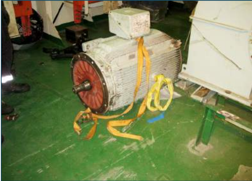
Figure 15: Electrical spare motor with broken lashings and damages from impact after having slid across the deck and hit other objects and structures. Source: Maersk A/S
