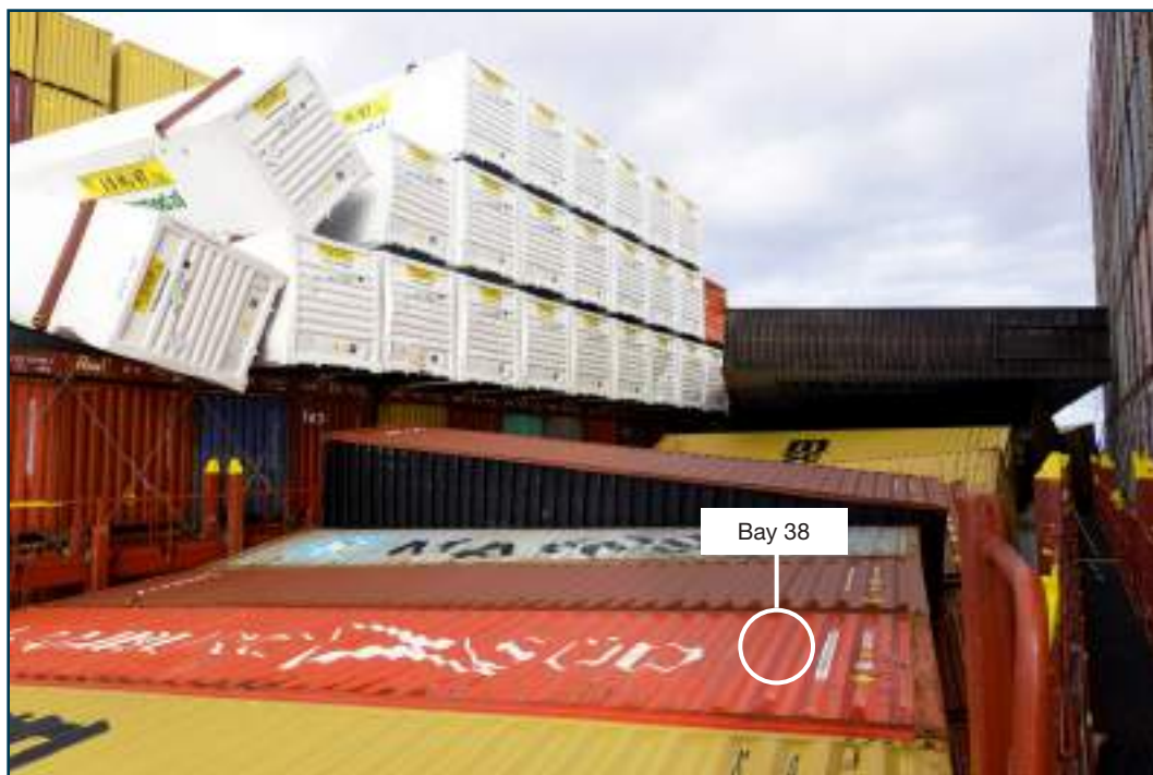
Figure 44: Bay 38 after the accident Source: Maersk A/S
