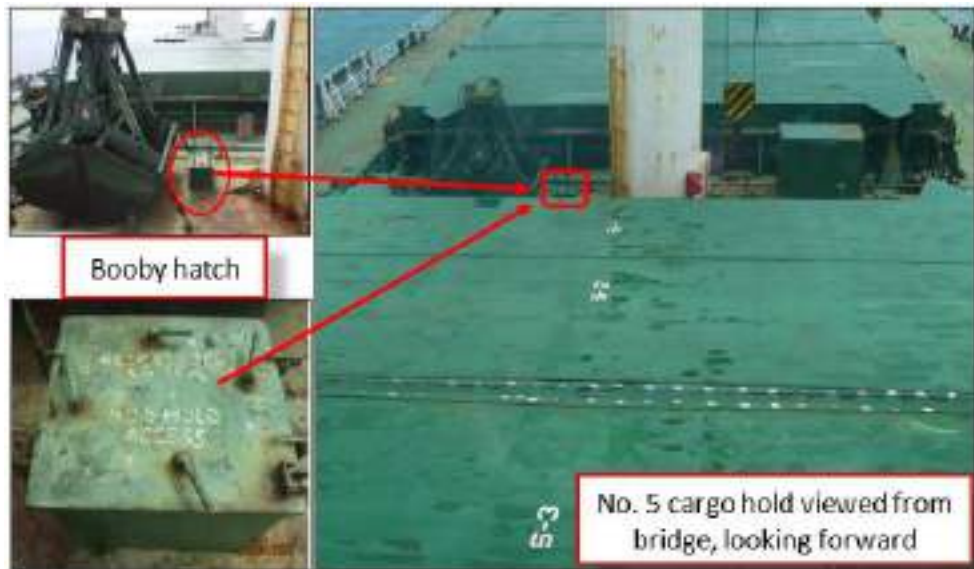
Figure 2 - No.5 cargo hold forward booby hatch - Source: the Company (Annotated by the TSIB)
