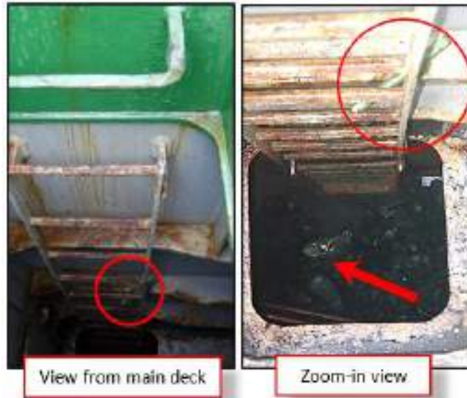
Figure 4 - Red-coloured circles indicating the dog handle and the arrow points to the safety shoes of ASD1 inside the cargo hold (Source: The TSIB)
