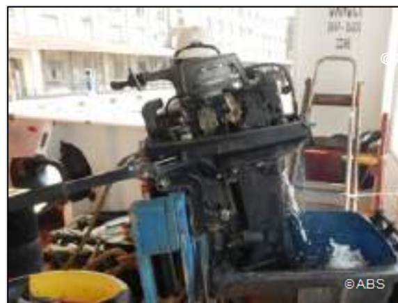
Rescue boat motor is not ready to operate due to cooling system out of order
