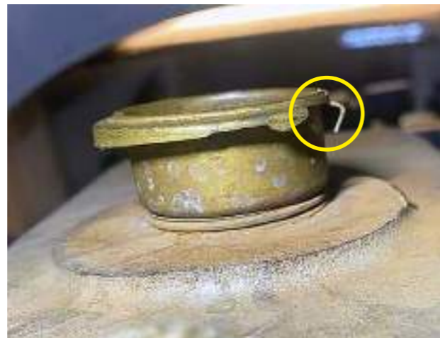
Figure 2: The bent securing lug
