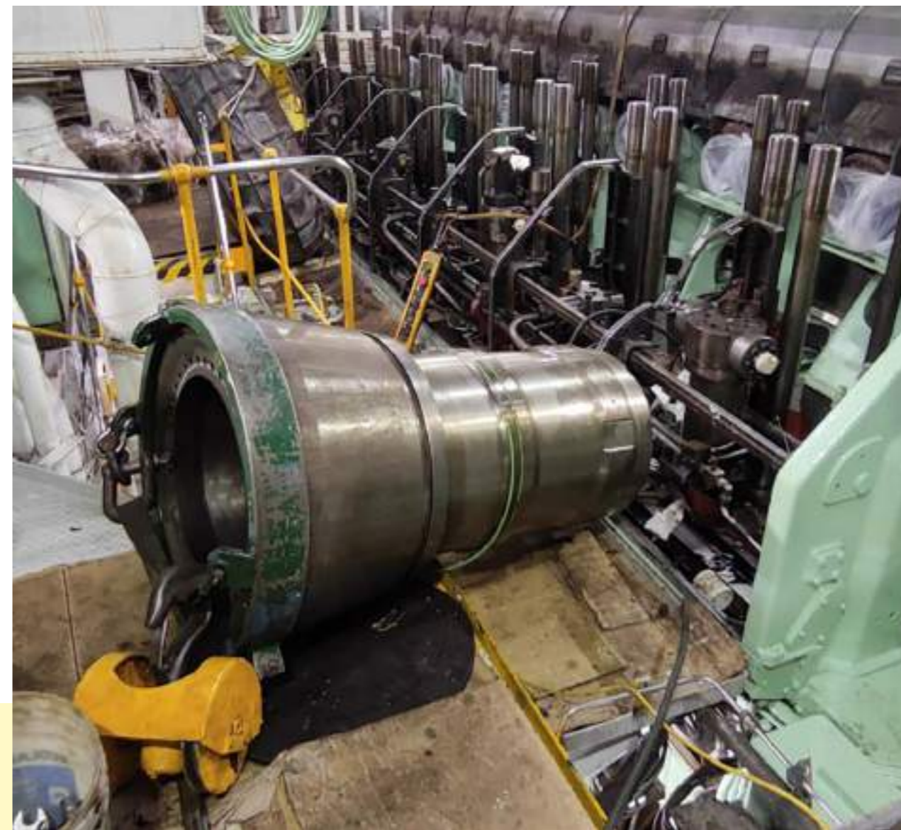
Figure 2: Position of cylinder liner after wire failure
