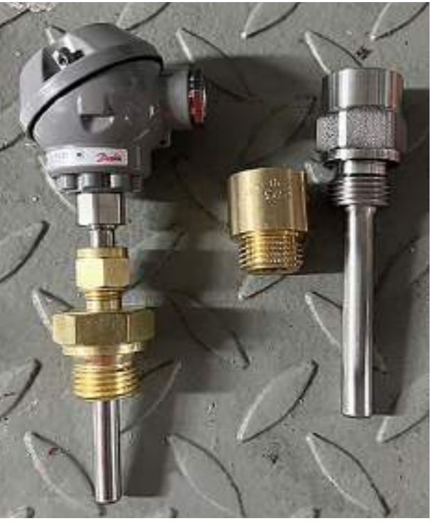
Figure 3: The new temperature probe fitting
