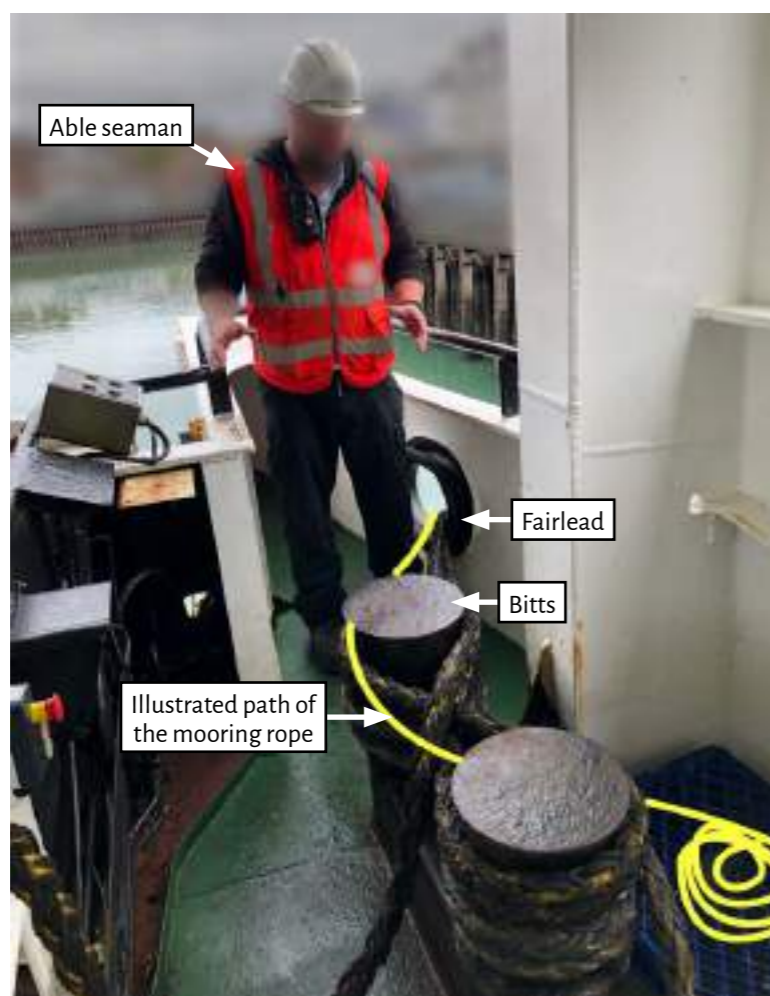
Figure 1: Reconstruction of the approximate position of the able seaman when he was struck by the mooring rope
