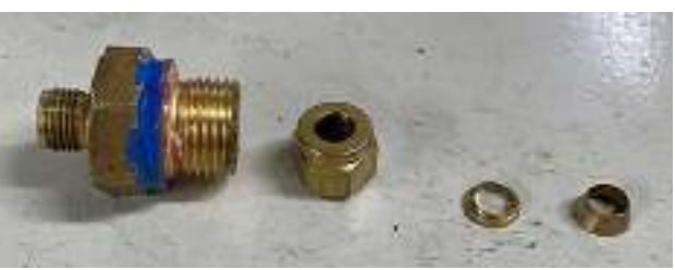
Figure 2: The original temperature probe fitting
