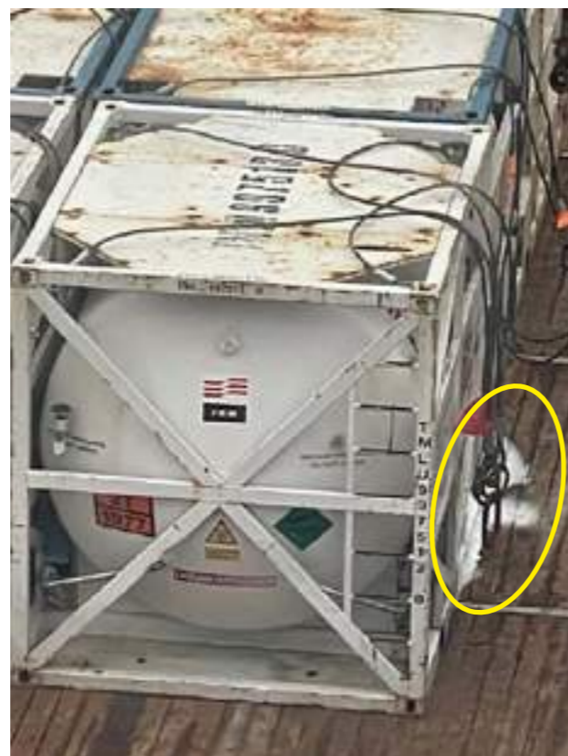
Figure 1: Icing of deck beneath nitrogen tank container
