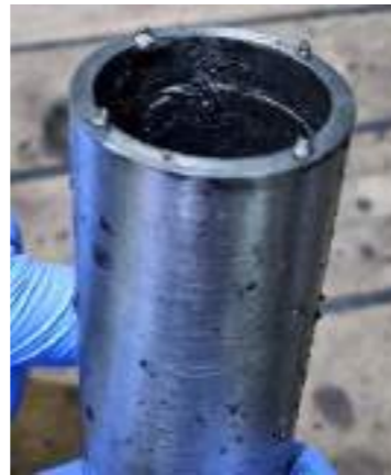
Figure 2: Water ingress and damage
