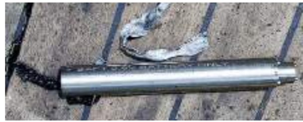
Figure 1: Damaged battery tube
