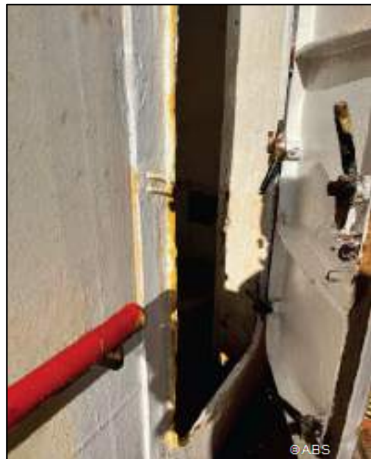
Weathertight door not closing, Gasket missing or edge wasted with knife-edge
