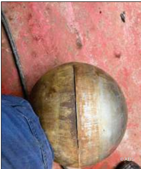
Tank vent head floater damage
