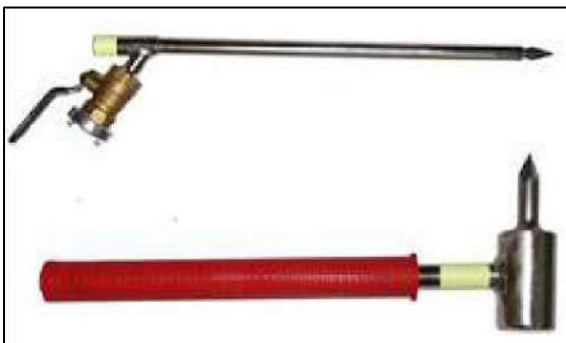
Figure 10: Fog lance kit, comprising of a water mist lance (the nozzle of which is designed to pierce a cargo container) and a penetration hammer (designed to punch a hole in a cargo container)
