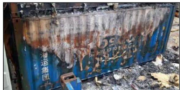
Figure 4: Container from where the fire originated (seen in its actual stowed position: 27-05-82)
