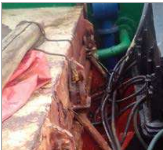
Hatch cover cleats not properly secured
