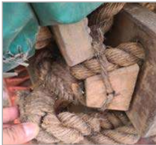
Embarkation ladders (Port and Star board) side rope wasted [Not properly maintained]
