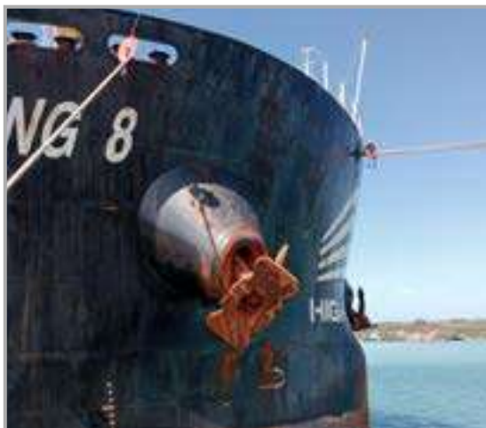
The Sea Anchor is much corroded [corroded]
