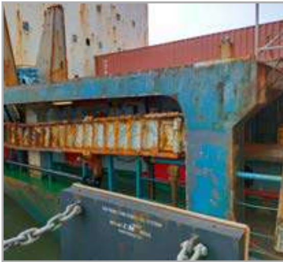
Accommodation ladder star board side found damaged [Damaged]
