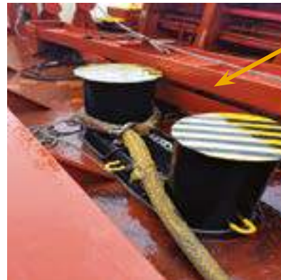
Log stanchion in lowered position
