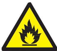
Flammable material or high temperature 1
