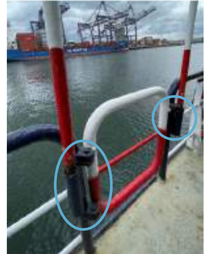
Figure 1: The poorly designed handhold stanchions (circled) that prevented the pilot from gaining a firm handhold
