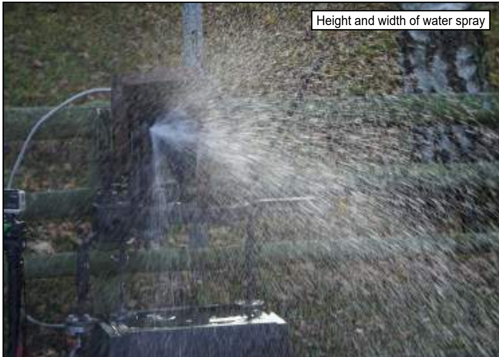
Figure 17: AE1 left-hand fuel filter leakage test
