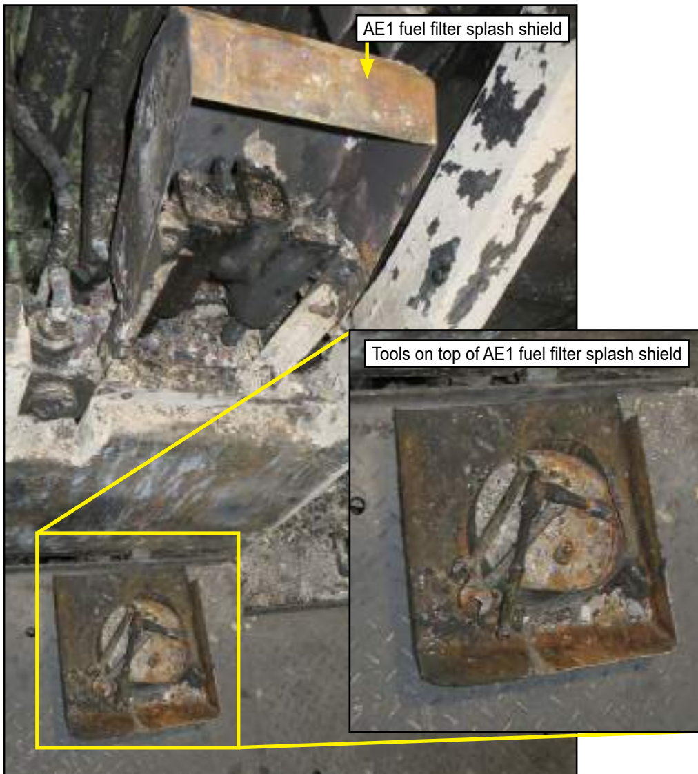
Figure 4: Post-fire AE1 fuel filter splash shield removed with tools on top
