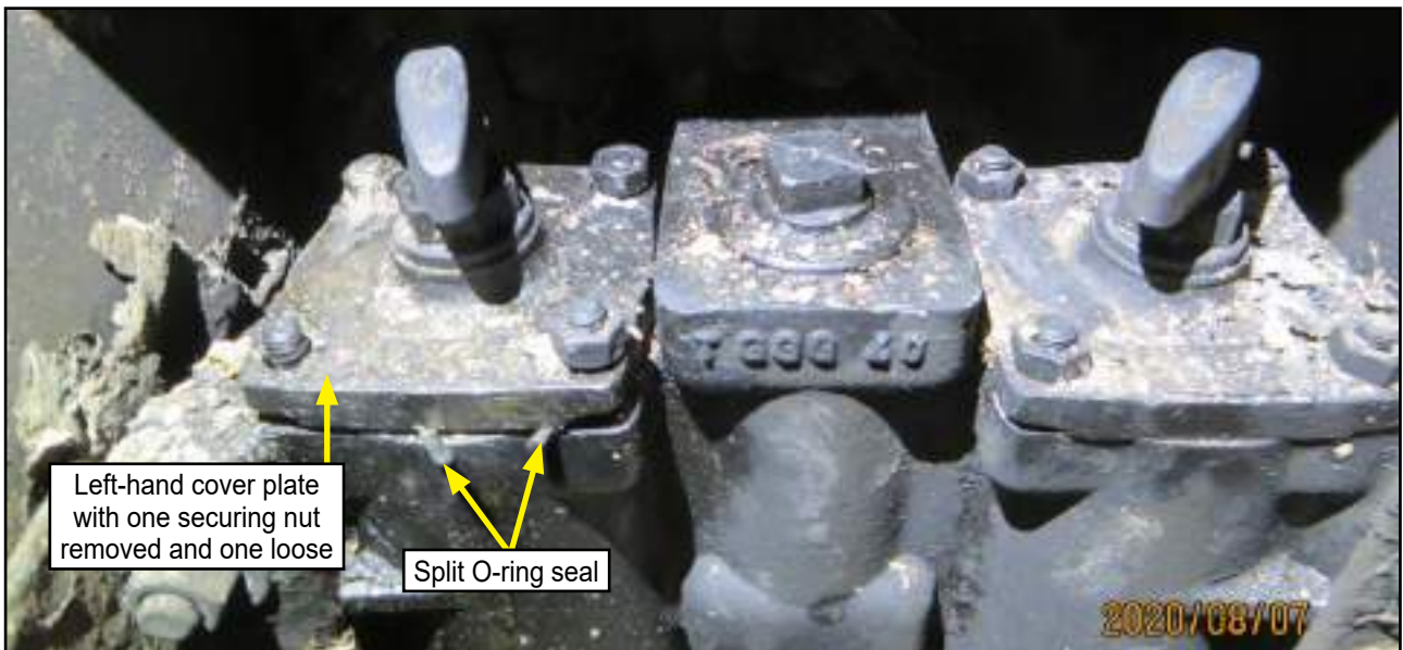
Figure 6: Post-fire AE1 fuel filters
