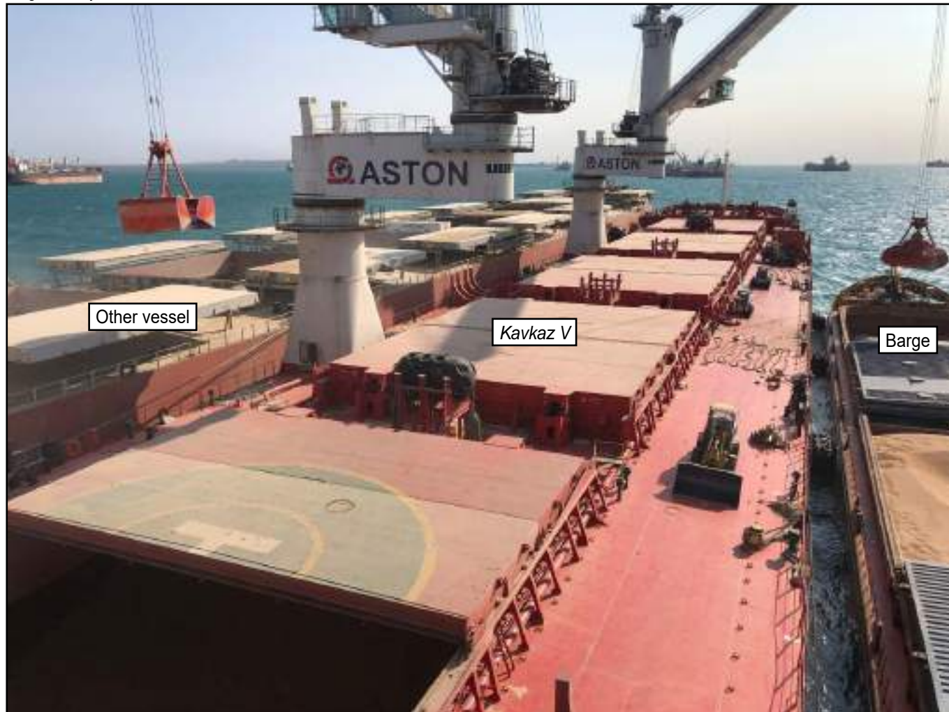
Figure 3: Kavkaz V (centre) loading grain from a barge (right) while transferring cargo to another vessel (left)
