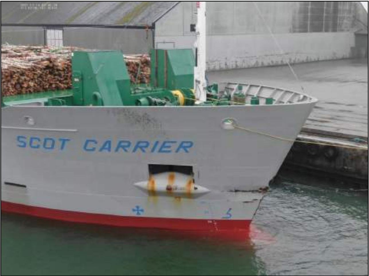
Figure 15: Damage to Scot Carrier's bow, showing collision damage on stem and hull, and silt staining above the ship's name
