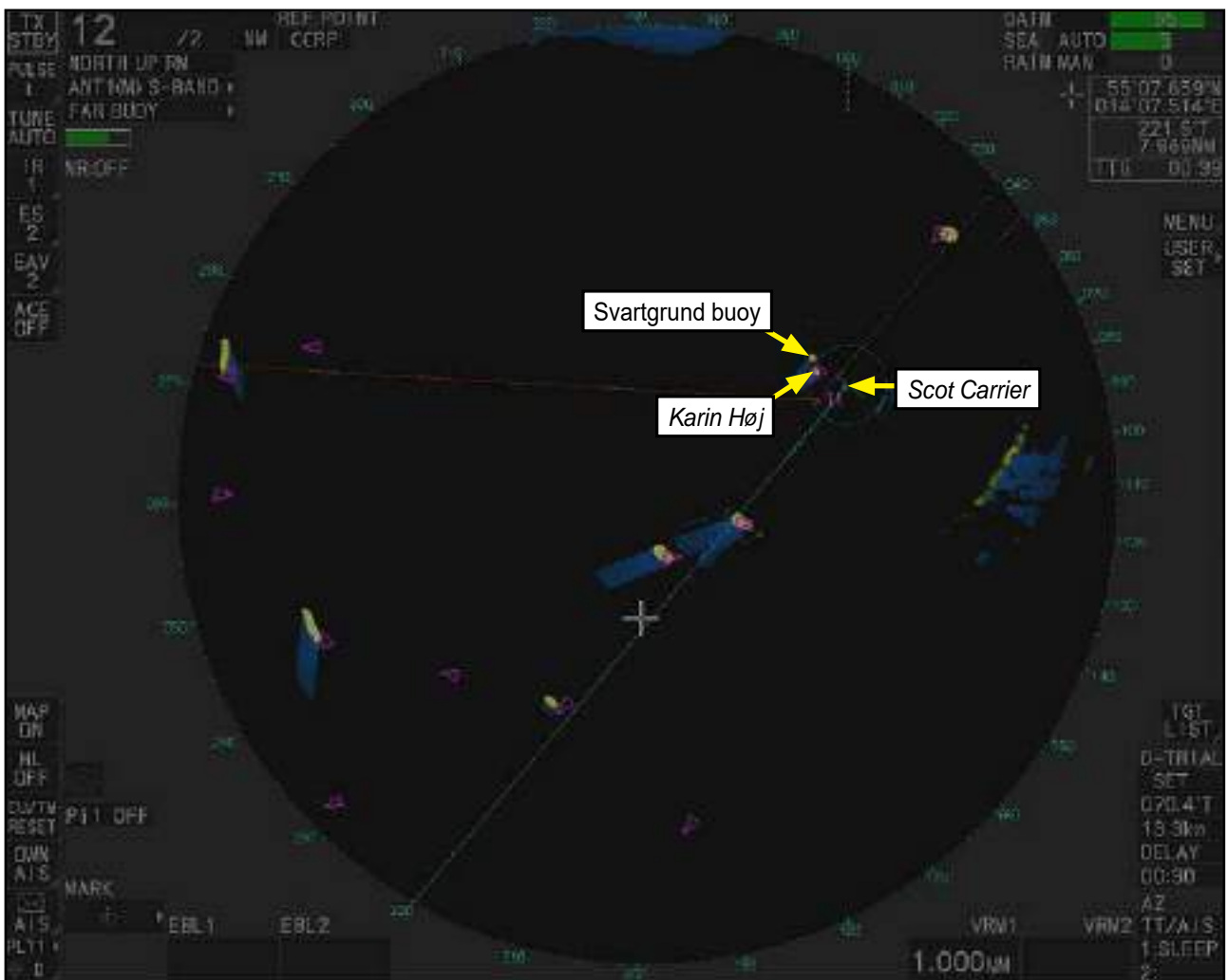
Figure 8: Scot Carrier's starboard radar image at 0321, before altering course
