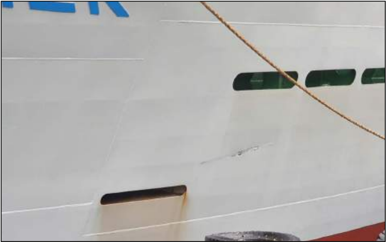
Figure 16: Damage to Scot Carrier's paintwork on the ship's port side
