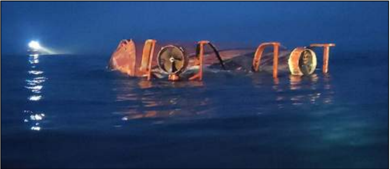
Figure 13: Karin Høj's upturned hull, showing azimuth drive units at the stern
