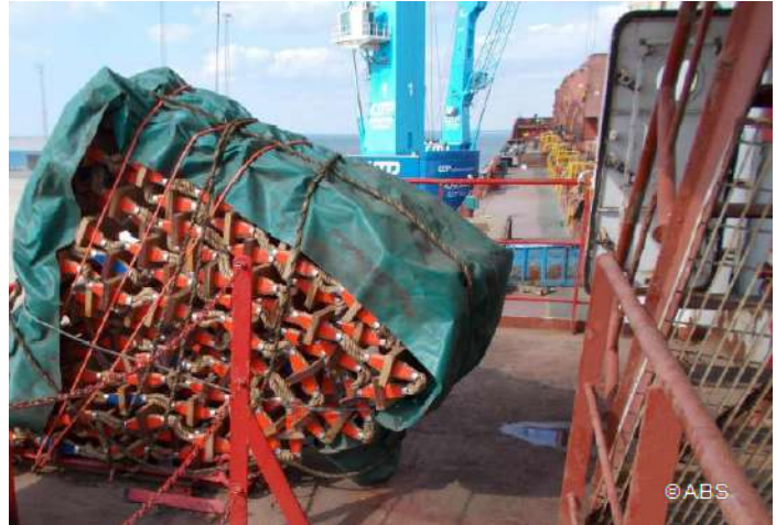
Improper stowage of embarkation ladder
