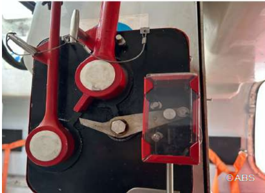
Lifeboat hydrostatic release not engaged and reset
