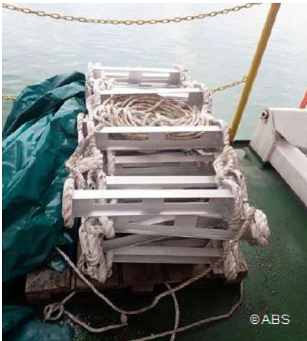
Non-compliant pilot ladder i.e., no rubber steps, loose chocks and retrieving lines not secured as required
