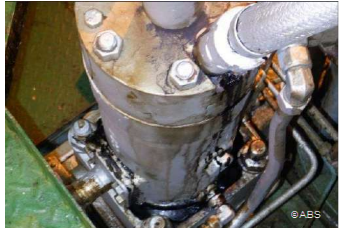
Main Engine Fuel Pump Leaking
