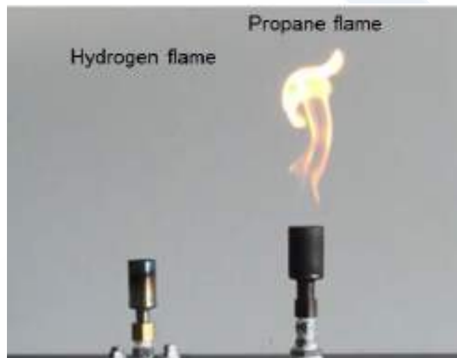
Figure 4 Comparison of a hydrogen flame and propane flame [19]
