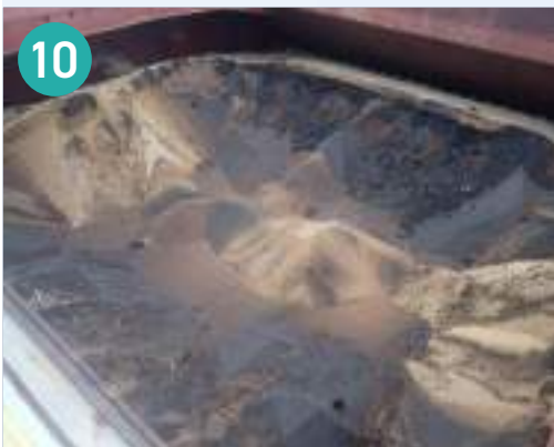
Figure 10: A severely heat damaged soya bean cargo with heavily blackened and carbonised beans.
