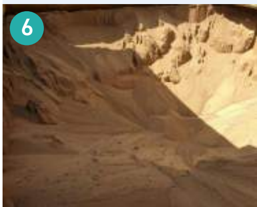
Figure 6: Partially discharged cargo of soya beans. The caking well below the cargo surface is indicative of mould growth between the beans causing them to stick together. The soya beans are only slightly discoloured at this stage.
