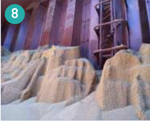
Figure 8: Soya beans caking well below the cargo surface in the lower part of a cargo hold. The caking indicates mould growth between the beans.
