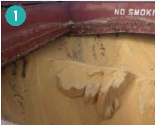
Figure 1: Mould residue on the hatch coaming from condensation wetting in a cargo of maize. Black, mould-damaged grains can be seen rolling down the cargo slope from beneath the deck areas where moisture condensed and wet the cargo. Cargo compaction/caking in the centre was due to prolonged stowage on board during a delayed voyage.
