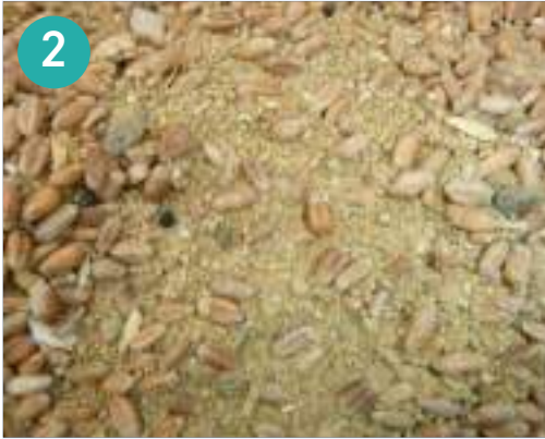
Figure 2: Cargo of wheat contaminated with a localised area of foreign material comprised of sand and stones. It is difficult to assess such contamination during loading due to the levels of dust and colour of foreign material.
