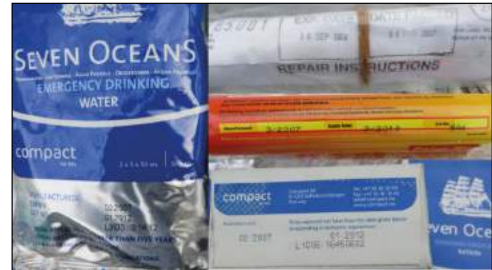
Figure 2: Examples of the expired consumable items in Piedras 's starboard liferaft
