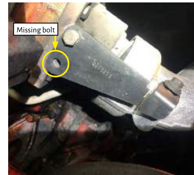
Figure 4: Fractured bracket and missing bolt
