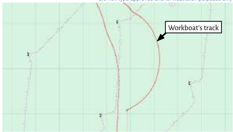
Figure 1: The navigational track of the workboat, showing its slow turn to starboard
