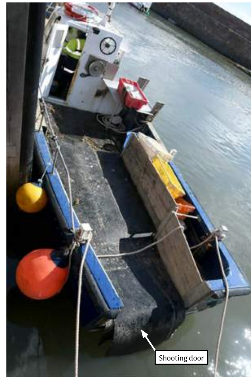
Figure 2: The shooting door (drop-in closing board removed)
