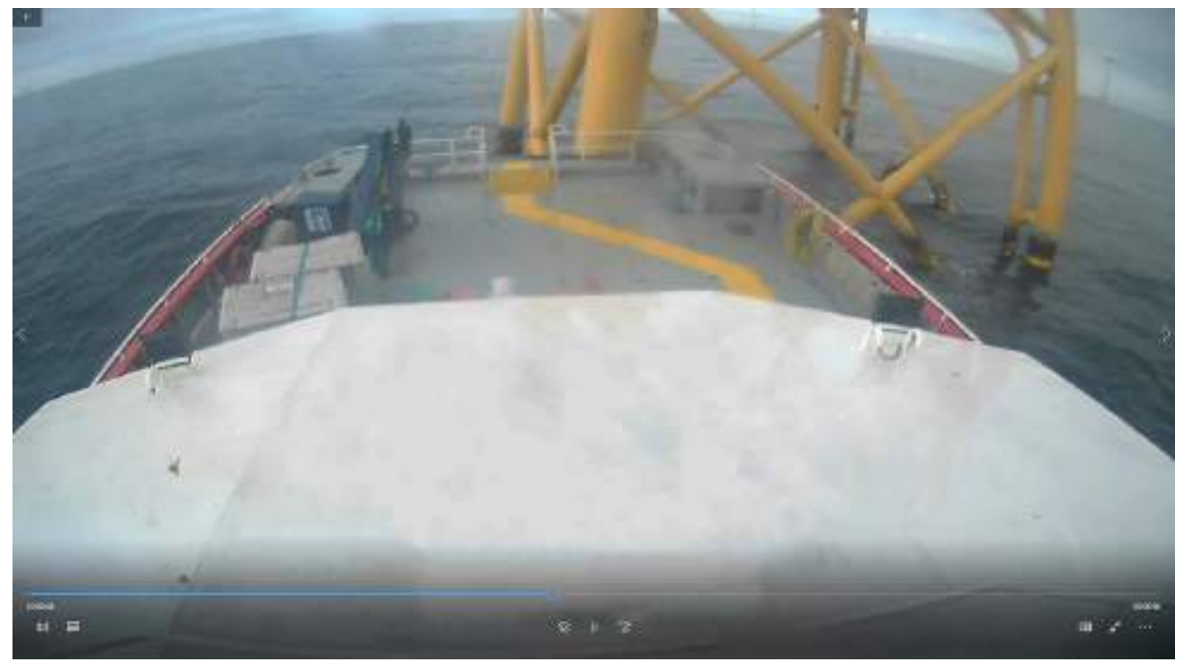
Figure 2: The moment the workboat bow collided with the wind turbine tower platform
