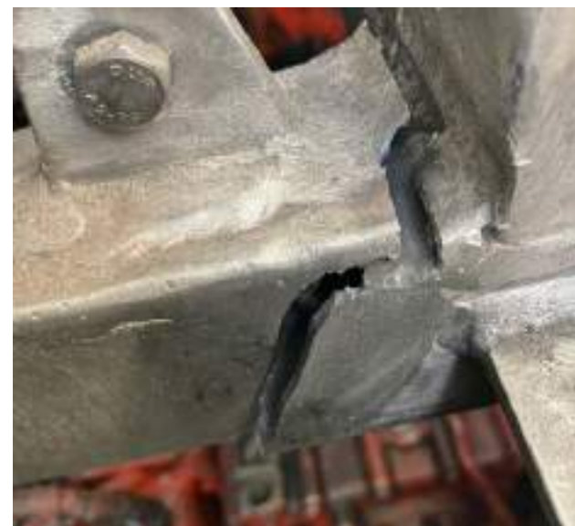
Figure 3: Fractured engine support
