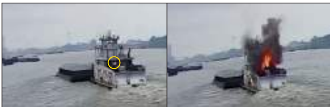
Figure 82. Above: Mary Lynn underway at 0652 on May 18, 2021, about a minute before the fire broke out. Below: Mary Lynn at 0652:40 (left) when the first open flame, circled in yellow, was visible on the second deck port side exhaust stack, and at 0652:45 (right).
