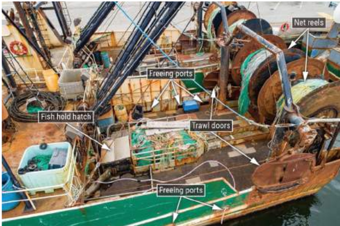
Figure 5. Aft working deck of vessel in 2019 before its purchase by Boat Aaron & Melissa. The storm gates are beneath the net reels and cannot be seen in the photo. BACKGROUND SOURCE: BLUE HARVEST FISHERIES
