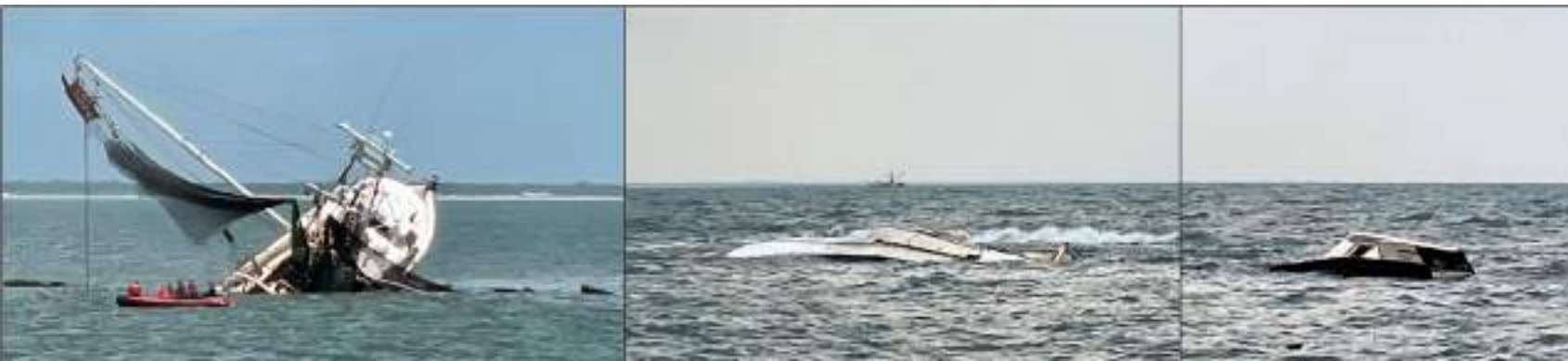
Figure 129. Left to right: Sage Catherine Lane following the grounding on the jetty, and after being broken apart on the jetty 3 days later.
