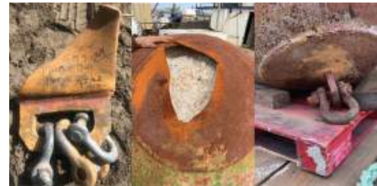
Figure 134. Left to right: SM-3 mooring buoy: failed weld (with three shackles) that separated from buoy; damaged top with padeye missing; and undamaged bottom padeye. SOURCES ALASKA MARINE SURVEYORS AND NORTHLINE SEAFOODS
