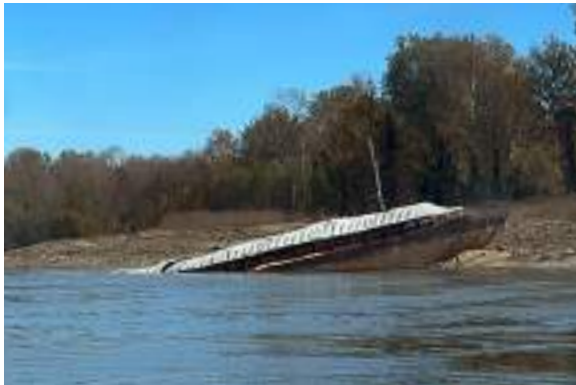
Figure 122. One of the Marquette Warrior 's barges that grounded and partially sank following the casualty.
