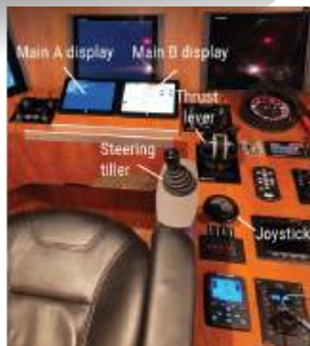
Figure 121. Commodore's main control station during postcasualty examination. Above: main A display screen's reboot failure (left) and the red failure log tab, red triangle over the port inner water jet icon, and the failure management pop-up screen on the main B display screen (right). Below: main control station's hand controls and water jet display screens.
