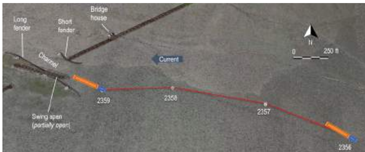
Figure 63. (Above) Trackline of the Robert Cenac , based on AIS course over ground data and the approximate position of the tow upon its contact with the Rigolets Bridge. Bridge position in the photo is about three-quarters of the way open. Tow headings are estimated. BACKGROUND SOURCE: GOOGLE EARTH
