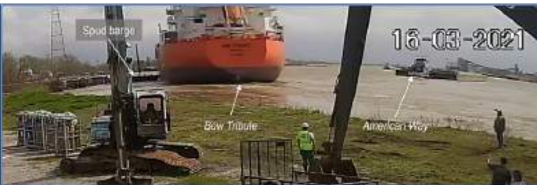
Figure 117. CCTV footage looking downriver at 1522:26 shows the Bow Tribute when it struck the spud barge protecting the New River water intake pipes.
