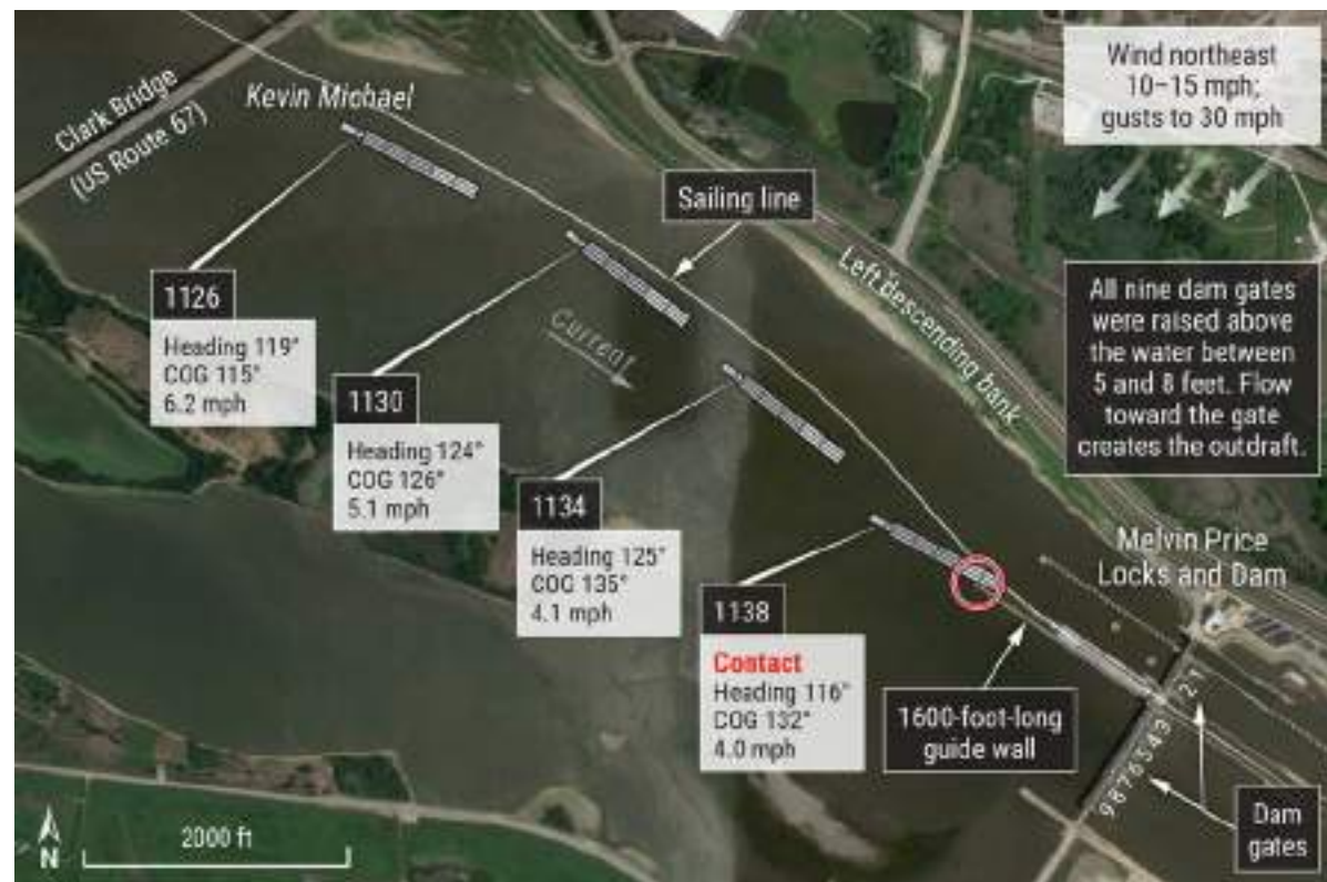
Figure 52. Annotated ECS track history of the Kevin Michael tow over the last 12 minutes leading up to the casualty. BACKGROUND SOURCE: GOOGLE EARTH
