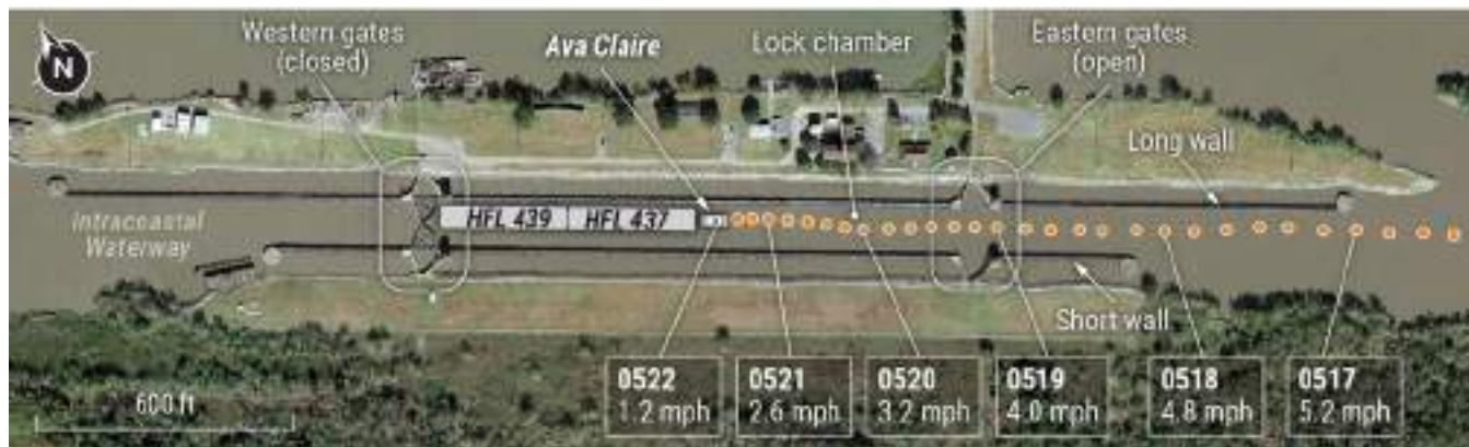
Figure 36. Automatic identification system (AIS) track of the Ava Claire , as indicated by the red dots, with a scaled representation of the tow added. The AIS antenna was located on the towing vessel, about 615 feet aft of the bow of barge HFL 439 . BACKGROUND SOURCE: GOOGLE EARTH.
