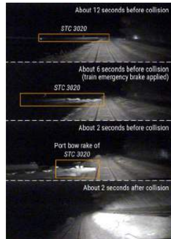
Figure 22. Still images of video footage from locomotive BNSF 9251's recorder as the train approached the barge and derailed after hitting the barge. The forward barge of the Baxter Southern tow is outlined in orange.
