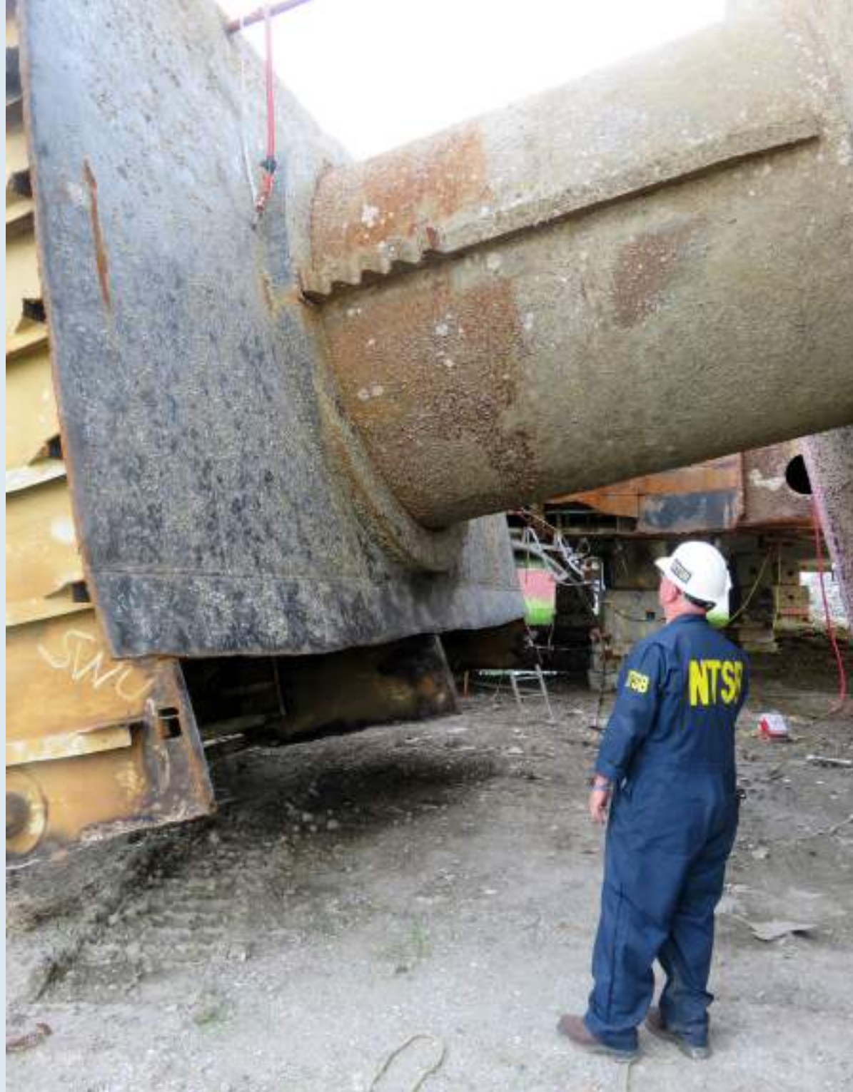
Figure 146. NTSB investigator Marcel Muise inspecting the SEACOR Power 's leg post-casualty.
