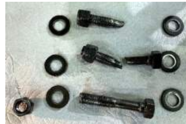
Figure 141. Damaged lower basket bolts, washers, and nuts from no. 3 engine's nos. 6 and 14 connecting rod and piston pair. SOURCE: WASHINGTON STATE FERRIES
