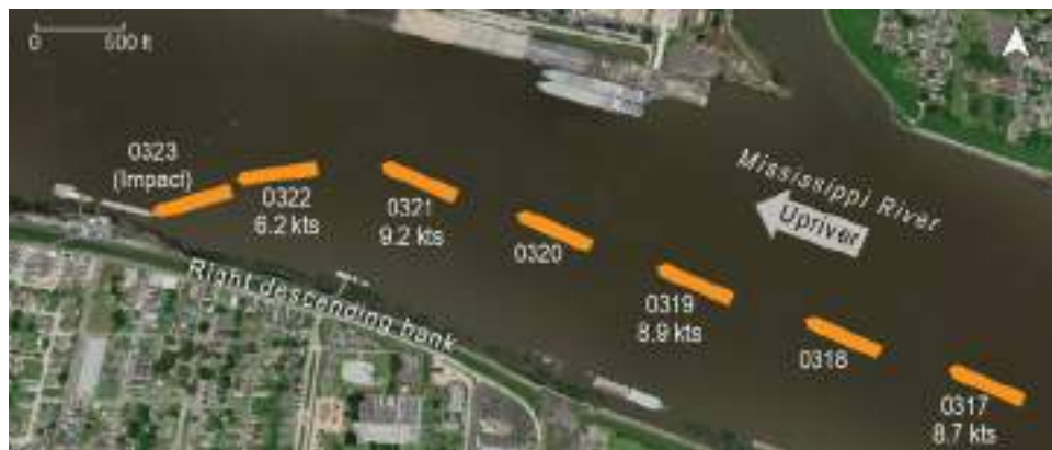
Figure 48. Left: Plotted positions of the Jalma Topic taken from the vessel's VDR from 0317 to the time when it struck the corner of the Smith's fleet office barge. Right: Smith's fleet barges and tug positions at the time of the contact. BACKGROUND SOURCE: GOOGLE MAPS
