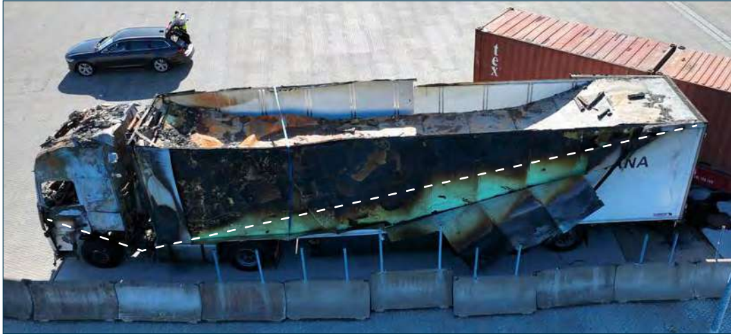
Figure 19: Fire pattern on the truck's left side. Source: DMAIB
