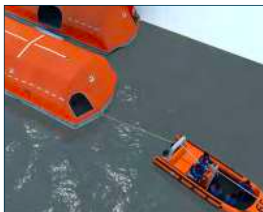
Figure 59: Additional raft being towed by FRB. Source: Viking Life-saving Equipment A/S
