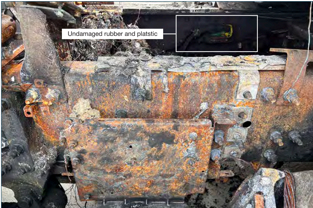
Figure 25: Undamaged plastic and rubber components on right-side chassis. Source: DMAIB
