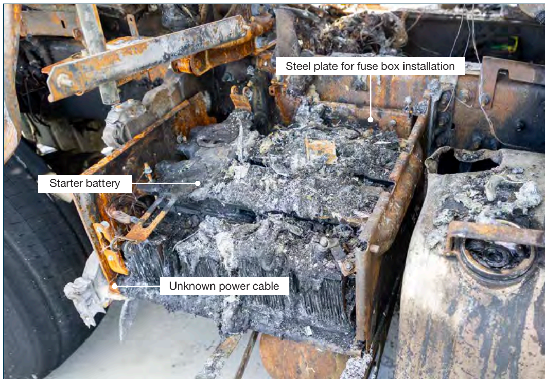
Figure 22: Starter battery mounted on the chassis. Source: DMAIB
