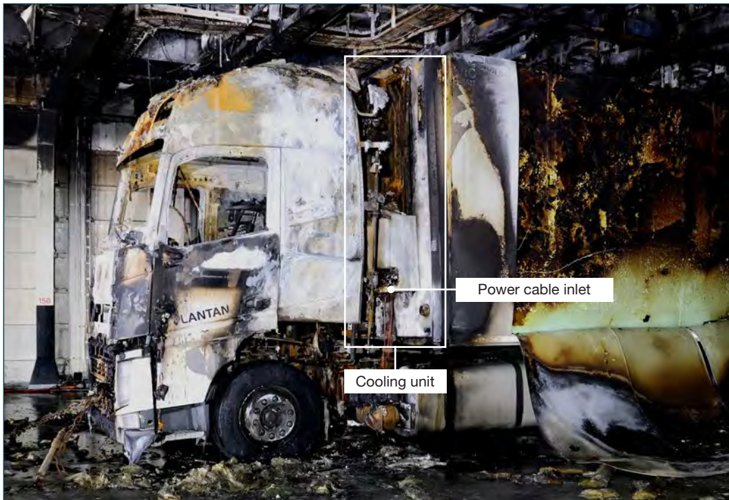
Figure 20: Fire damaged cooling unit. Source: DMAIB
