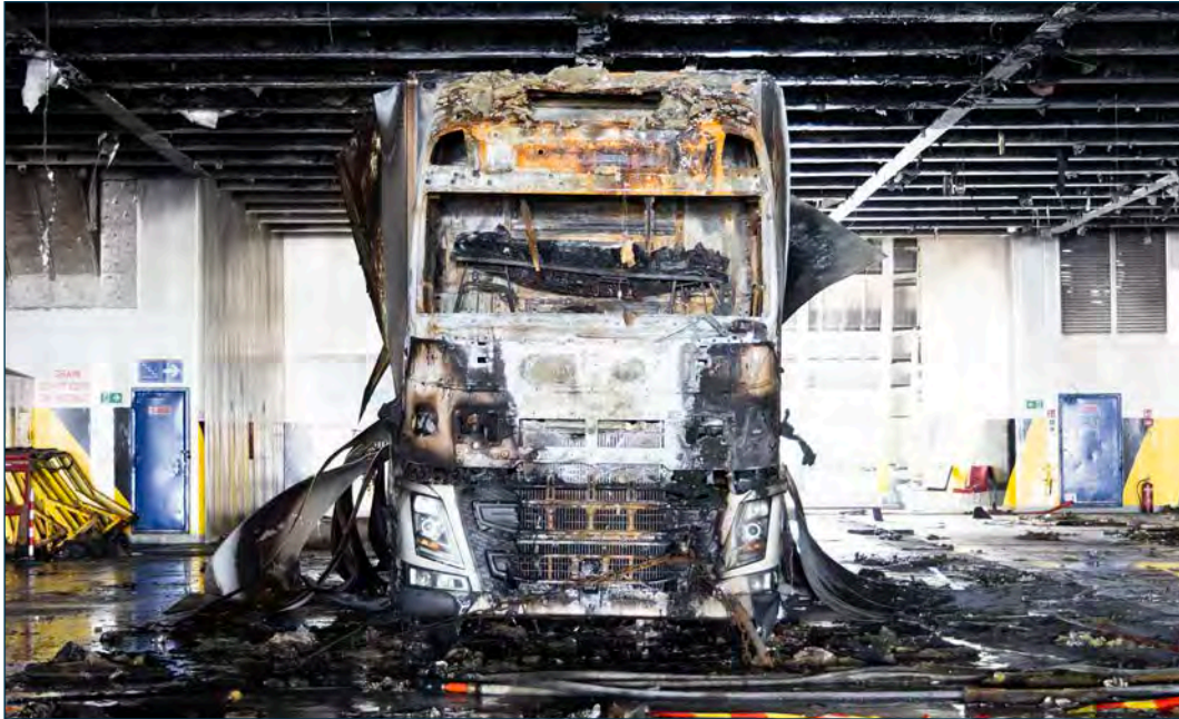
Figure 17: Fire damages on truck front. Source: DMAIB
