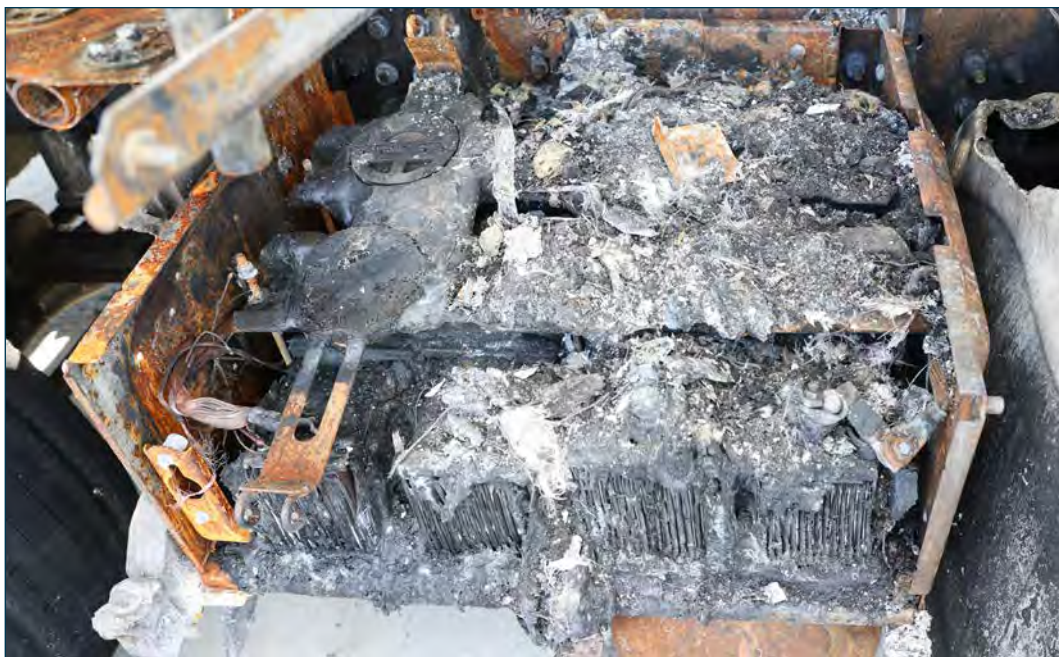
Figure 27: Damaged starter battery. Source: DMAIB
