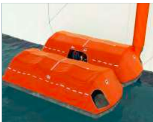
Figure 58: MES with additional raft launched. Source: Viking Life-saving Equipment A/S
