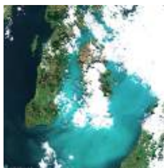
Sentinel-2 MSI image of the Clyde Sea on 21 June 2021 11:35 UTC, True Colour with enhanced contrast. Processed by NEODAAS, using ACOLITE atmospheric correction.
