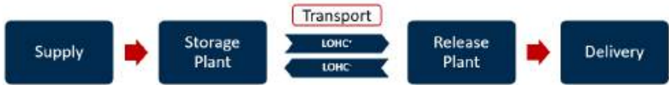
Figure 6. Example showing the process flow of the LOHC value chain by Hydrogenious LOHC Technologies. A plus refers to bonded hydrogen, a minus refers to hydrogen that is not bonded in the LOHC molecules.
