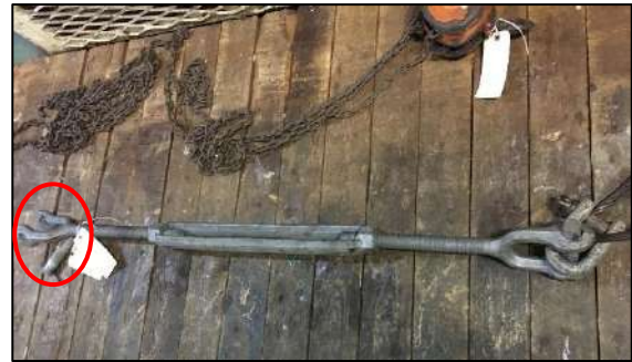
Figure 7: Photograph of the turnbuckle with the securing pin out of place at one end (red circle)
