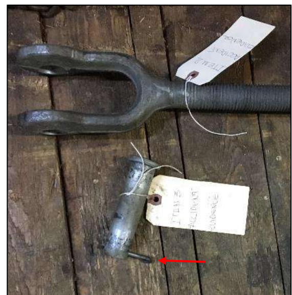
Figure 8: Close-up photograph of the turnbuckle with the securing pin (red arrow: split pin in place)
