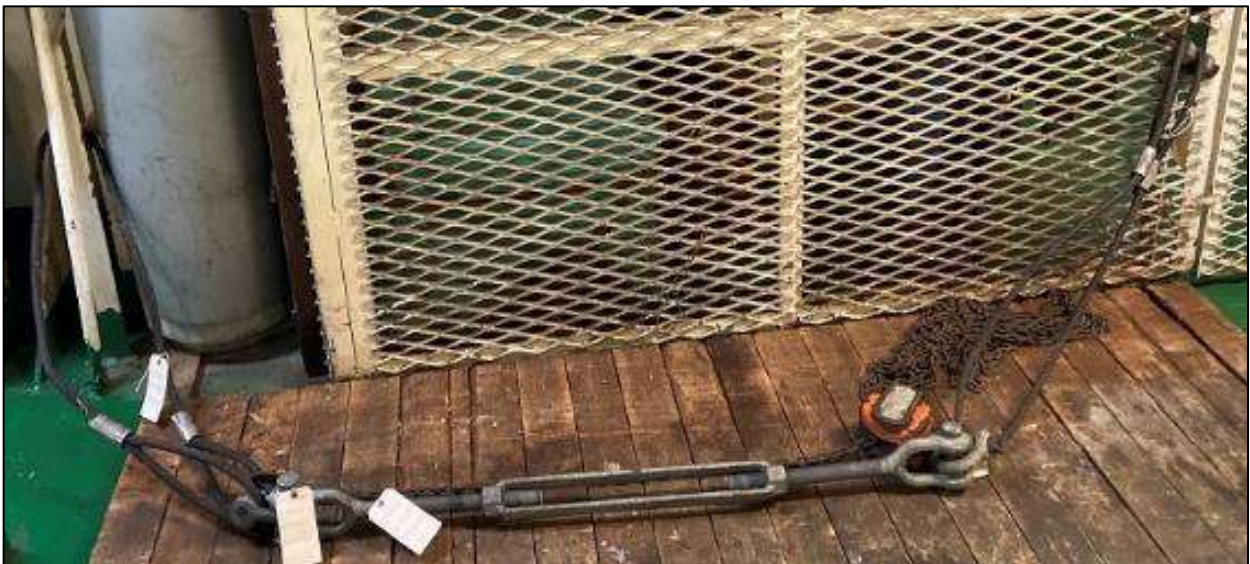
Figure 5: Simulated photograph of the securing arrangement
