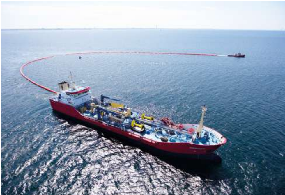
Stand-by Oil Spill Response Vessel Norden during a drill with oil boom deployment.
