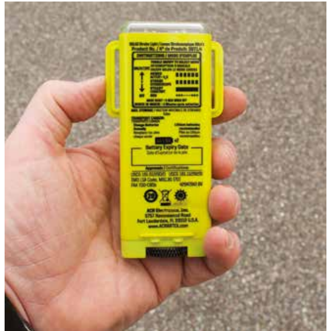
A typical personal locator beacon (PLB)
