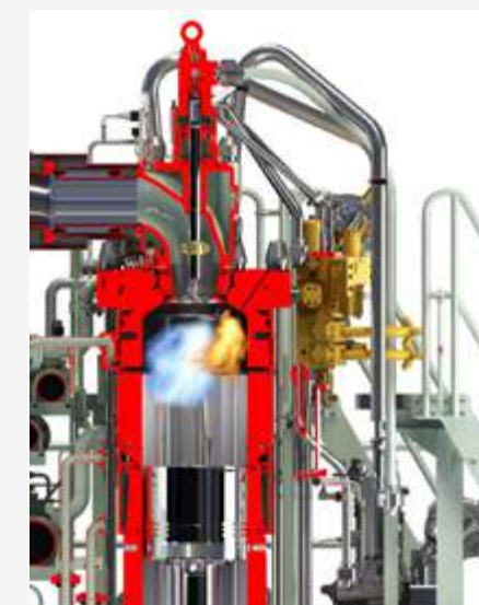
MAN ES ammonia dual fuel cylinder cross-section
