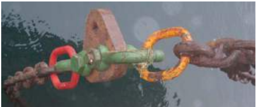
Figure 22 Emergency towline rigged for a barge
