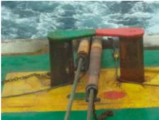
Figure 17 The use of two tow wires
