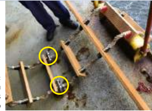
Figure 2: A pilot ladder reported in 2023, showing the shackles against the step
