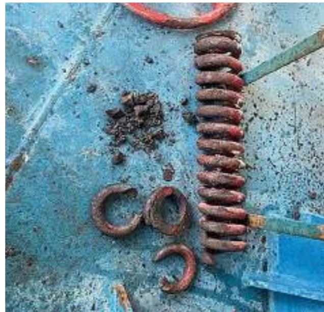
Figure 2: The broken anchor cable brake spring
