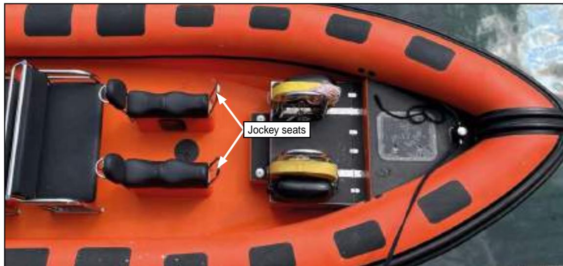
Figure 1: Front of RIB with jockey seats
