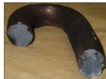
Figure 2: Failed chain link on Honeybourne III
