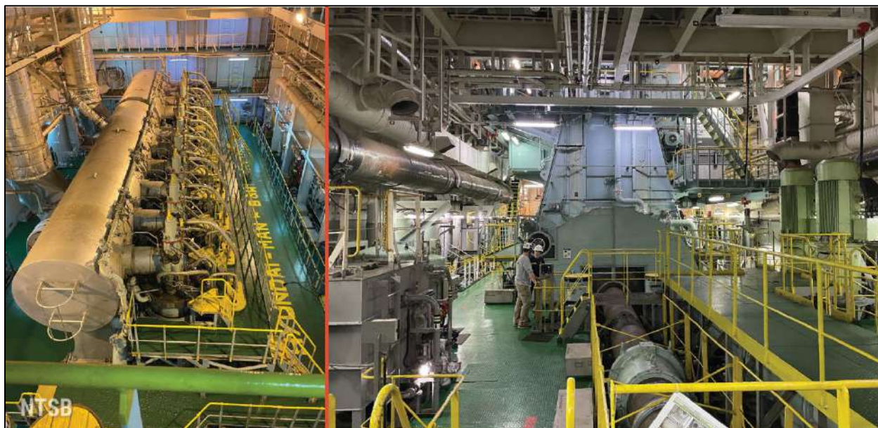
Figure 2. Left: The Dali 's main engine room (looking aft), showing the vessel's engine. Right: NTSB investigators examining the lower level of the vessel's engine room (looking forward).
