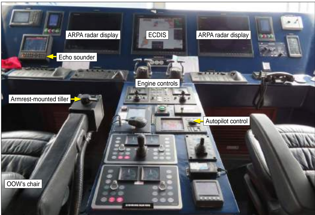
Figure 2: Central OOW console, showing the layout of steering controls and navigational equipment
