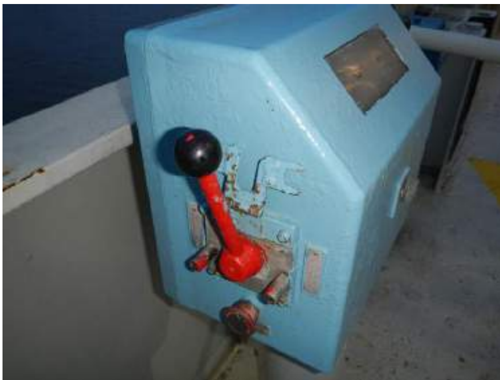
Photo 2: The picture shows the maneuvering lever. By putting a loose piece of equipment it was forced locked into high-speed position. Photo: SHK.
