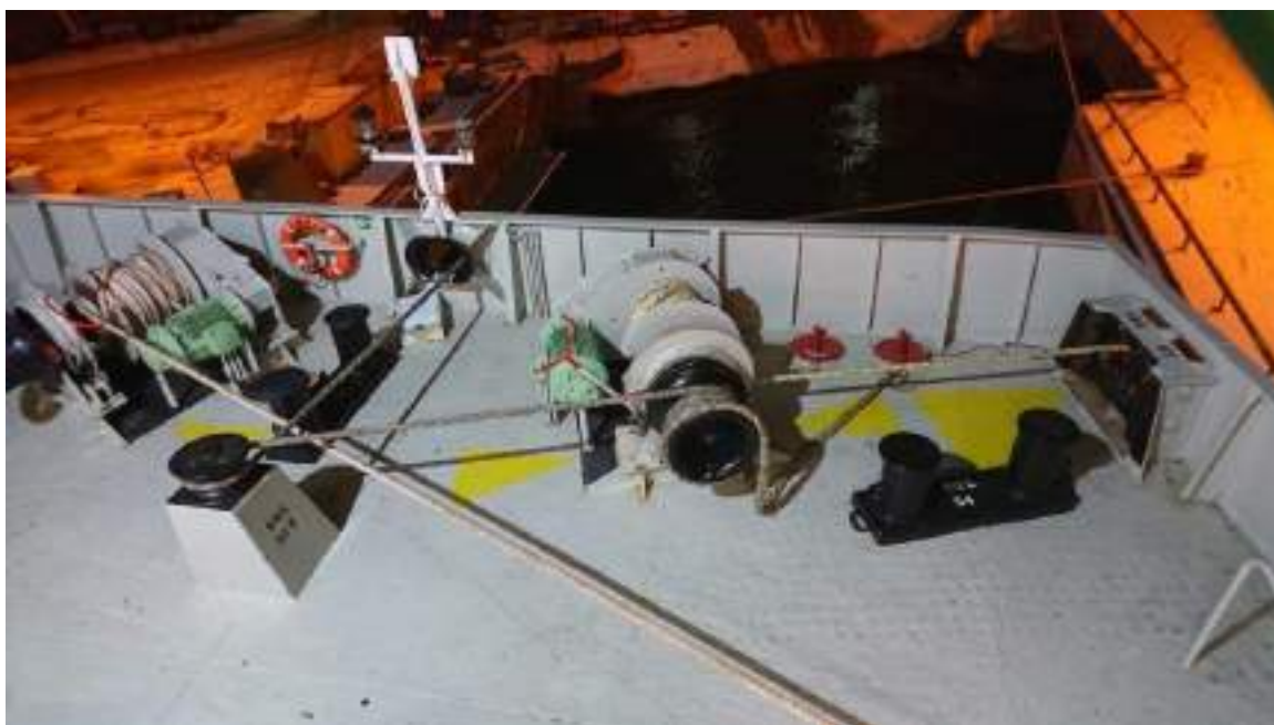
Photo 1: Image from the accident scene. In the very center, the black drum with the extra rope is seen. In the deck, towards the quay, two small red hatches are seen. The extra rope was to be put through one of these. Photo: SHK.
