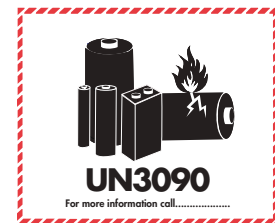
Lithium Battery Mark § 173.185(c)(3)
