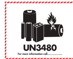
Lithium Battery Mark § 173.185(c)(3)
