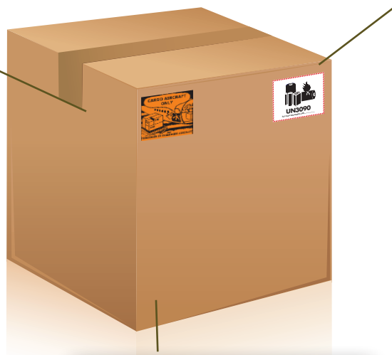
Lithium Battery Mark § 173.185(c)(3)
