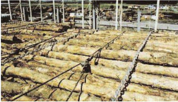
Figure 14.7: The correct use of wiggle wires through snatch blocks, which are used to bind and consolidate the log stow and are independent of the number and pitch of cross lashings required. Photo shows chain cross lashings pitched 3 m apart for a stow not exceeding 4 m in height above the weather deck at the ship's side.
