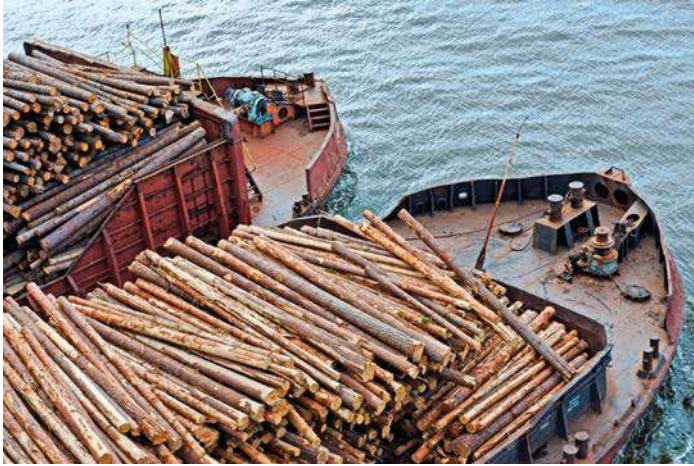
Figure 14.4: Timber cargo poorly stowed and improperly secured.
