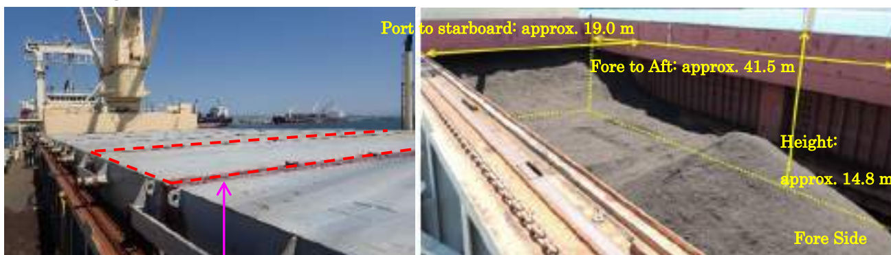
The hatch cover is divided into multiple sections.
