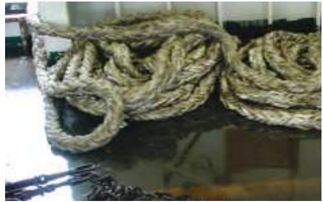
Ropes badly stored on wet deck
