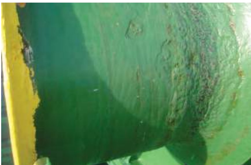
Build up of paint on the drum end
