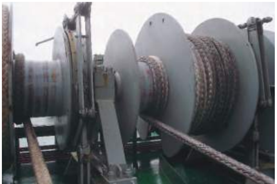
Correctly set up split drum
