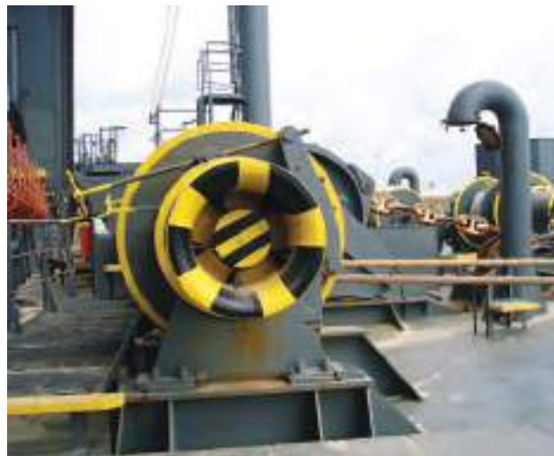
Mooring station with effective hazard markings
