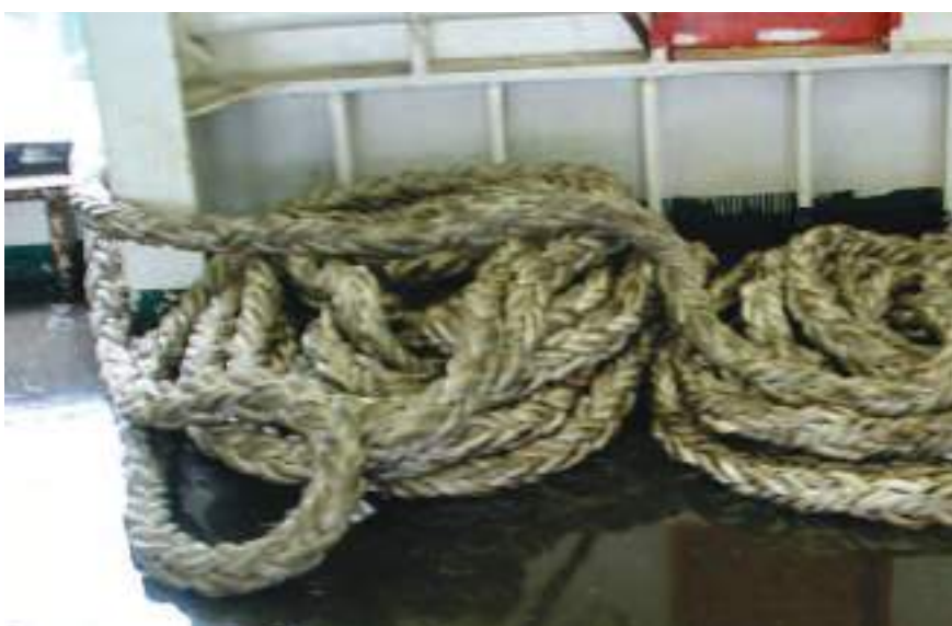
Ropes badly stored on wet deck
