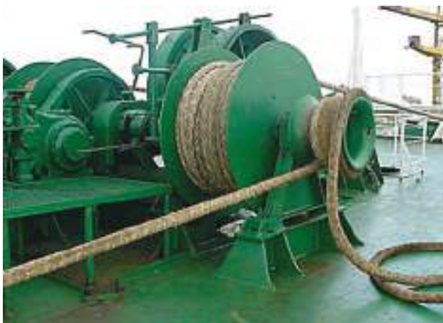
Well painted but poorly highlighted mooring station
