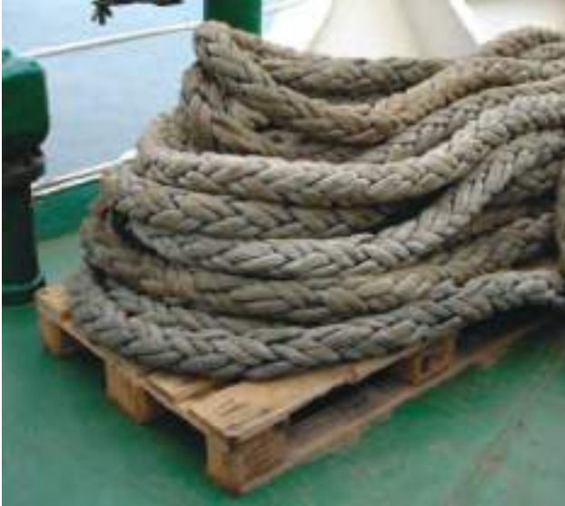
Ropes correctly stowed off deck
