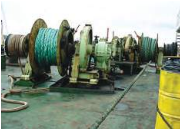
Mooring station with effective hazard markings
