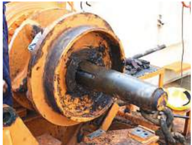
This windlass drum suffered bearing damage and is being overhauled
