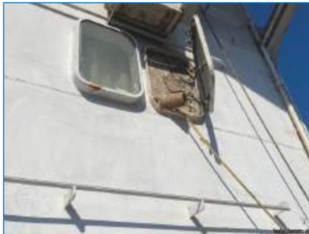
Non ship type air condition hose passing through cabin window on starboard side.
