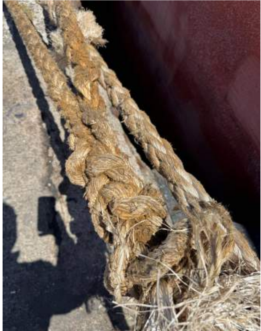
Mooring ropes in poor condition
