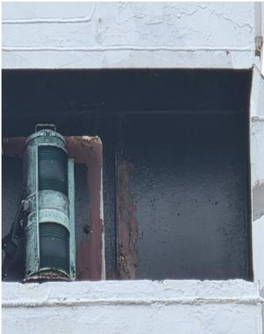
Starboard navigation side light screen is not painted fully in matt black, which may cause light reflection and impair visibility, contrary to COLREG 72 Annex I, Section 9(a)(i).
