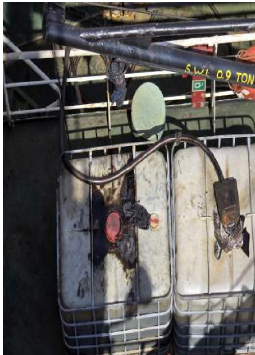
Oil storage tanks with transfer line keep on poop deck
