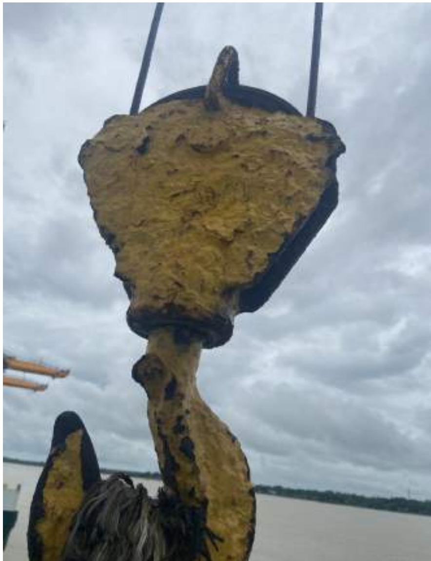
Provision crane 's block was found rusty condition and not proper mark for SWL
